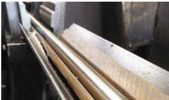
Through-feed centerless grinding for bar stock
